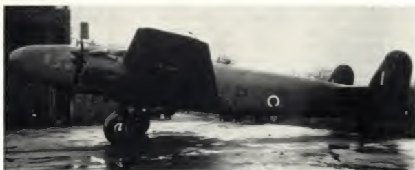
L9515 in Dark Green/Dark Earth/Yellow prototype finish. She was the trials installation aircraft which led to the Mk II Series IA. Here she features the revised nose, has a flattened four gun dorsal turret and lengthened nacelles—all features to improve performance. Photograph was taken in the winter of 1942-43.
